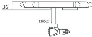
Note: When mounted with a magnetic mount, the vehicle may only be driven at low speed. If the vehicle is driven at high speed, the warning light bar may come loose and cause damage. It is the driver's responsibility to drive the vehicle at a suitable and safe speed.
